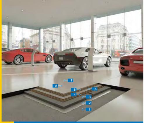
13 System for the installation of ceramic tiles without tracing the pattern of existing distribution joints
