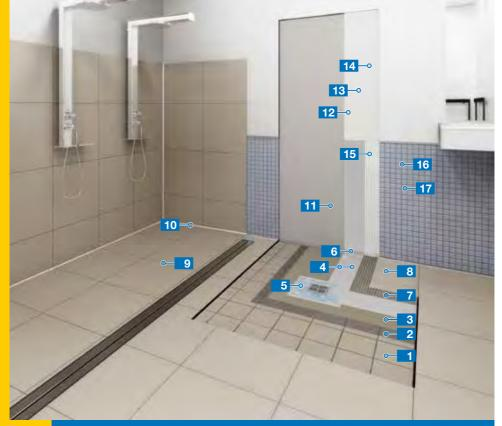
System for waterproofing and bonding ceramic in shower booths, bathrooms and changing rooms by overlaying existing flooring
