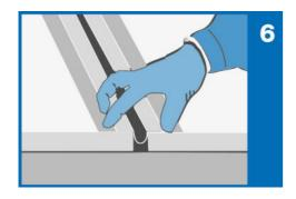
Butt joints between two strips of **Mapeband TPE** must be carried out by overlapping and bonding at least 5 cm of the central part in TPE by either hot-welding or cold-welding, as illustrated previously. To make the welding of the parts in TPE easier and firmer, press lightly with a flat carpeting roller (fig. 9).
