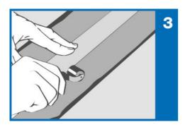
Apply a second layer of **Adesilex PG4** while the first one is still fresh, completely covering the fabric strip with the new layer of adhesive (fig. 4). Smooth off the product with a flat trowel.
