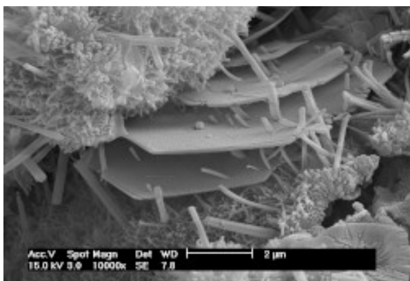
Hydration of a Portland cement-based binder in a traditional grouting mortar
