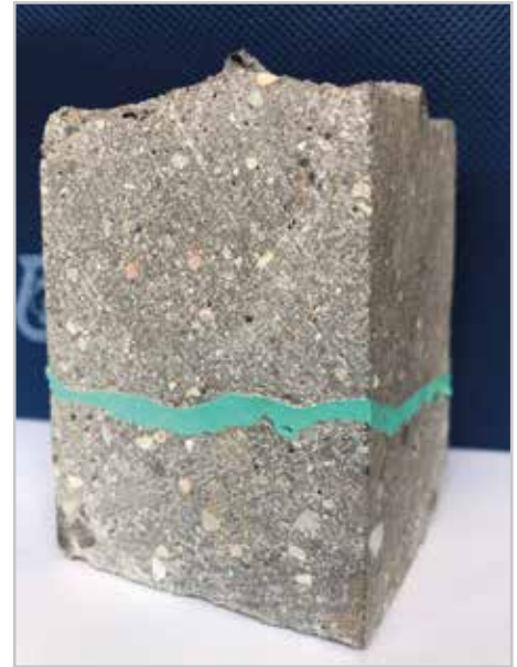
MAPELASTIC TU SYSTEM composite lining (“sandwich” system)
