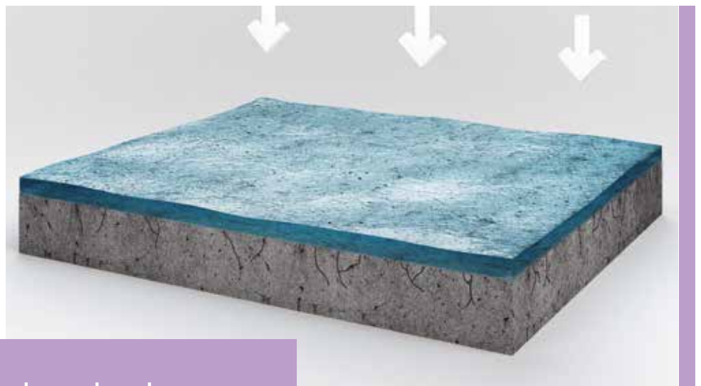
Photo 2 Idrocrete KR 1000 reacts with water to fill microcracks with crystalline deposits
