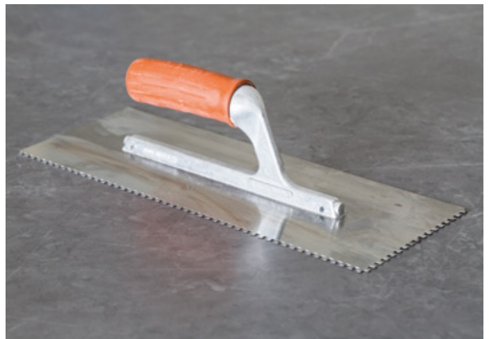
A spreader with sloping notches to spread the adhesive on the substrate and with square notches to spread the adhesive on the back of the tile
