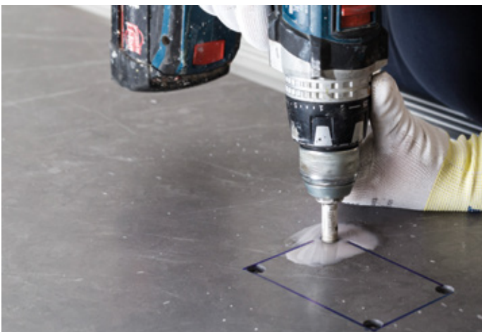
Sequence to make a rectangular hole
