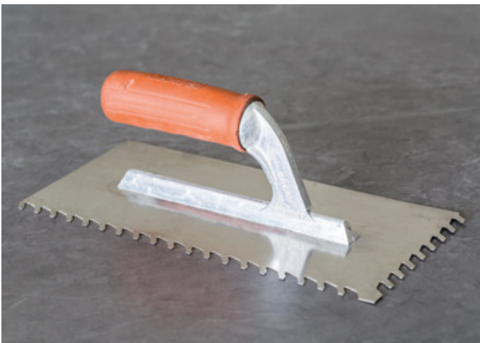
A spreader with sloping notches to spread the adhesive on the substrate and with square notches to spread the adhesive on the back of the tile
