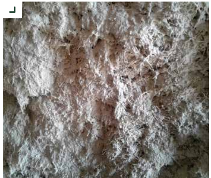
Enlargement of the fibres in PLANITOP INTONACO ARMATO
