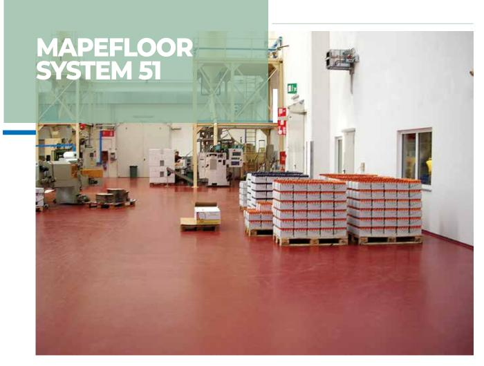
Multi-layered vapour-permeable epoxy system in water dispersion with a matt non-slip finish for industrial floors; average thickness 3 mm.
