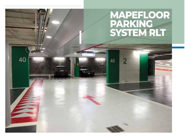
Multi-layered, seamless epoxy system for pedestrian surfaces and areas with vehicle access exposed to intense traffic. The system complies with Rili DafStb (Guidelines of the German Committee on Reinforced Concrete) OS 8 and the concrete surface protection systems according to EN 1504-2; thickness 0.8 to 1.2 mm.
