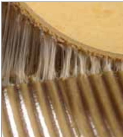
Fig. 4.4 - The legs effect of adhesives with high initial tack
