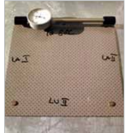
Fig. 4.10 - Instrument used to measure dimensional stability (after accelerated ageing) according to EN 1903 standards: on the left a free covering, on the right a bonded covering
