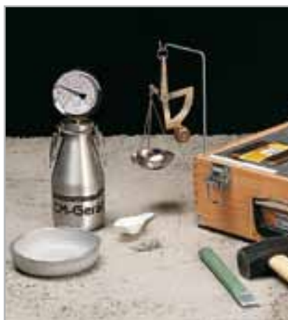
Fig. 3.4 - Carbide hygrometer used to measure residual humidity in screeds
