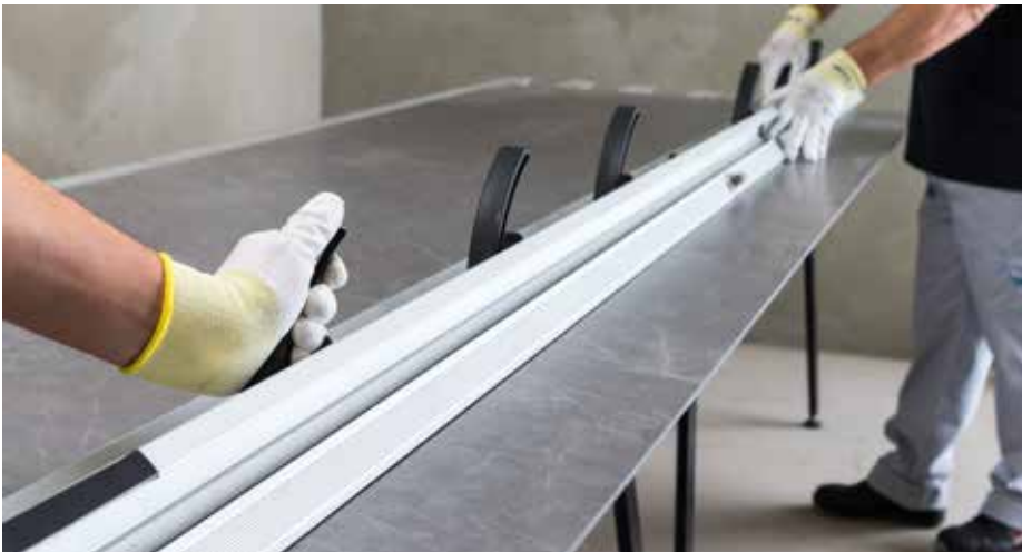
Cutting guide to make a straight cut
