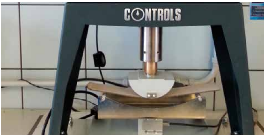
Measuring the deformability of cementitious adhesive
