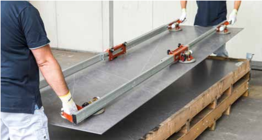
Correct handling of a tile
