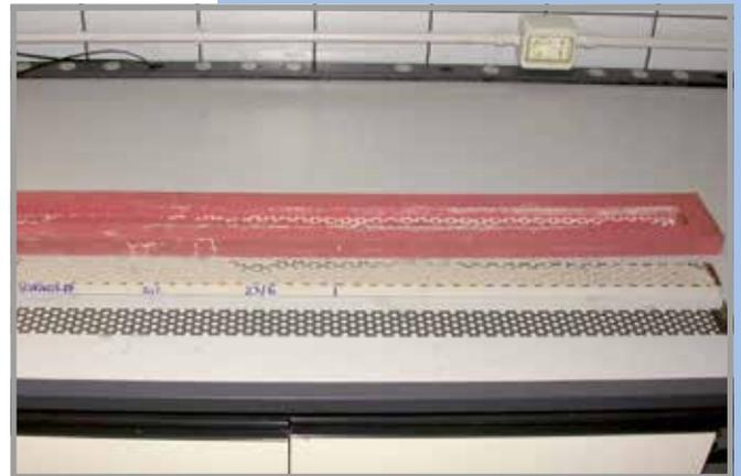
However, the method described above only allows dimensional variations of the samples to be measured after hardening, and does not allow the behaviour of the product during the plastic phase to be monitored. It is during this phase that the product is subject to higher transformation of its mechanical properties, passing from a fluid state to a solid state.
