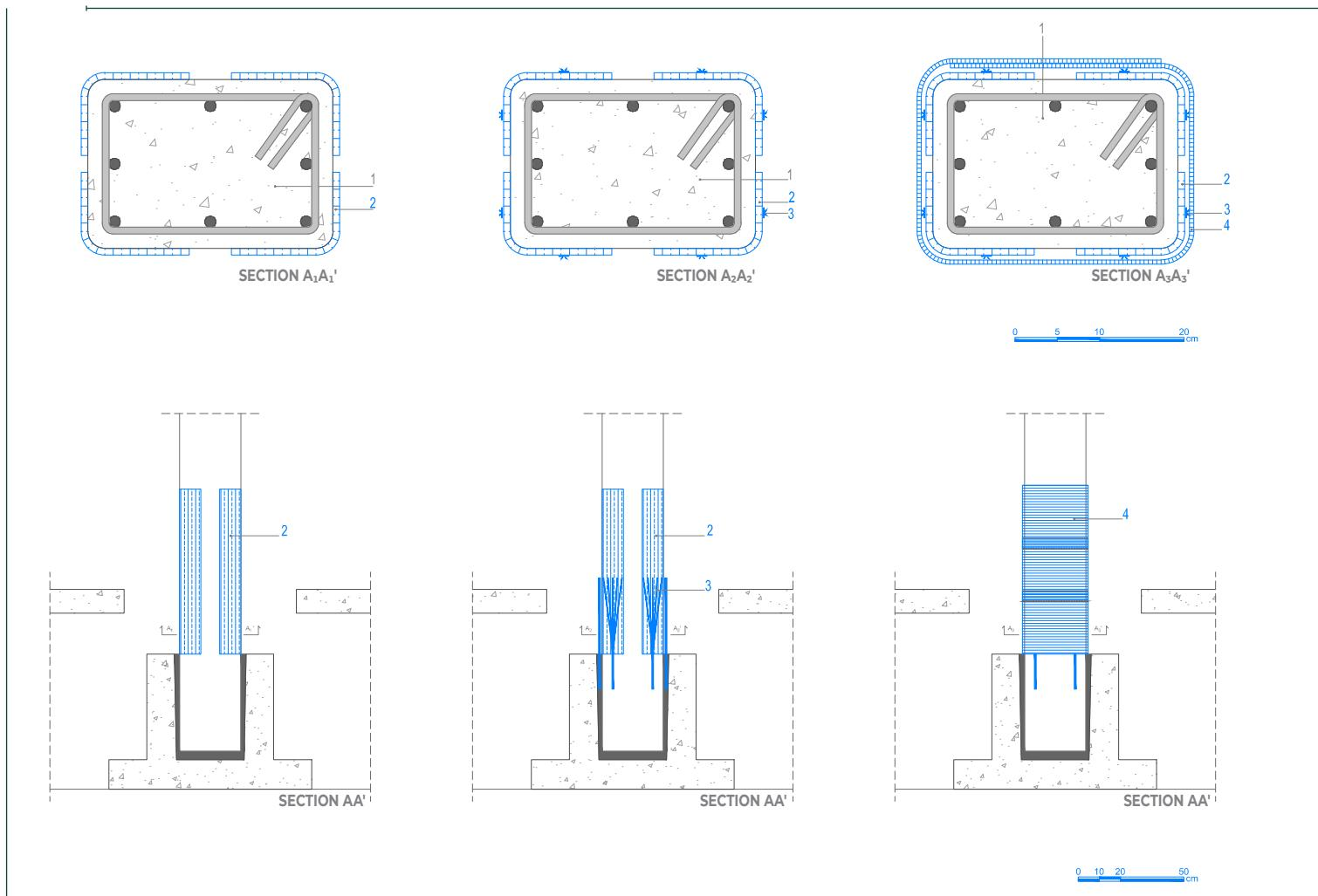
the pillar at right angles to the longitudinal axis of the pillar. Go over the fabric with a **MAPEWRAP ROLLER** to eliminate any air bubbles. The sheets and strips of fabric must be applied so that there is always an overlap of 20 cm in a horizontal direction and 5 cm in a vertical direction (photo K).
