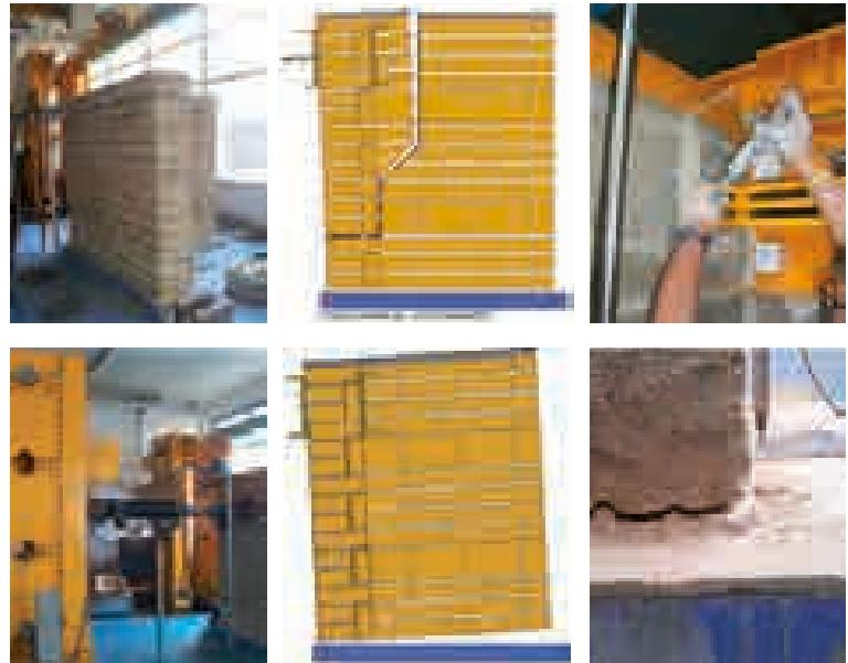
"T" intersection to dissipate more energy than the test piece without strengthening, and without any significant modification to its initial rigidity, and prevent the collapse mechanism that had been observed in the test piece without strengthening.
