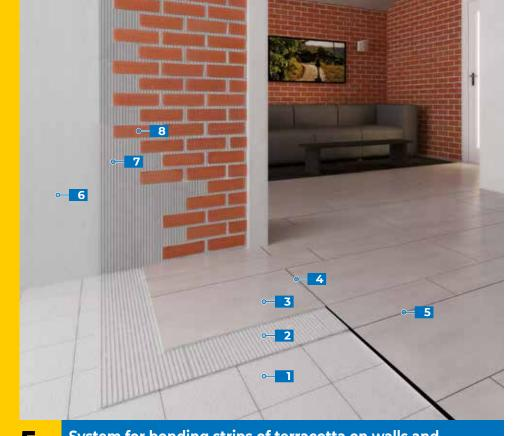
System for bonding strips of terracotta on walls and overlaying porcelain tiles on existing floors
