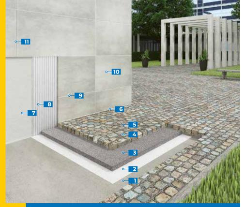
System for bonding large, thin ceramic tiles on façades and installing porphyry block flooring
