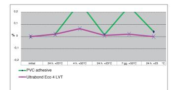
Results of dimensional stability tests carried out on an LVT strip according to EN 1903 standards with Ultrabond Eco 4 LVT compared with a generic adhesive for PVC.
