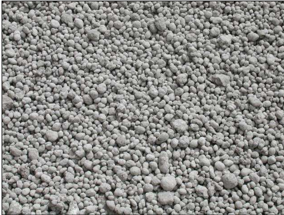
Figure 2. Artificial granular aggregates obtained with the proposed S/S process. The diameter of the largest grains is approximately 16 mm.
