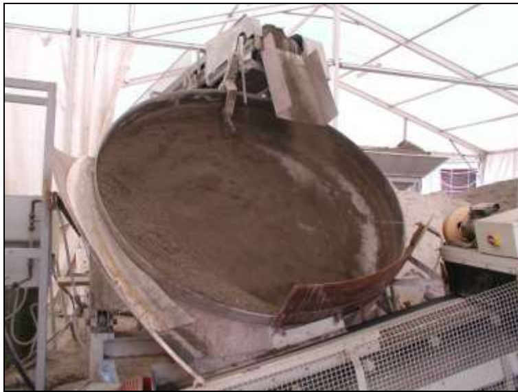
Figure 1. Rotating plate apparatus used for the pelletization process of the aggregates. Diameter of the plate: ~ 3.5 m.
