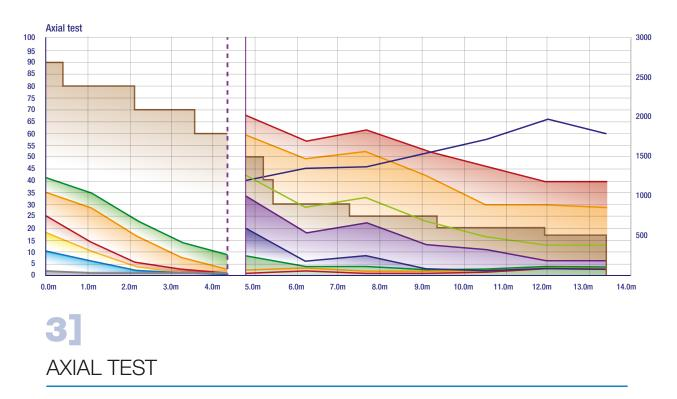
This procedure allows the plant to verify the performance and if necessary to adjust the ball charge. It is very useful to perform the Axial Test before the planned maintenance period. In this case it is possible to adjust the ball charge after analysing the results.
