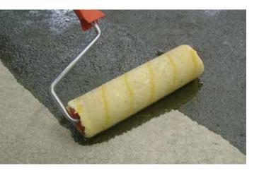
One-component solvent-free moisture-hardening polyurethane primer with very low emission of volatile organic compounds (VOC) for consolidating and waterproofing cementitious screeds.
