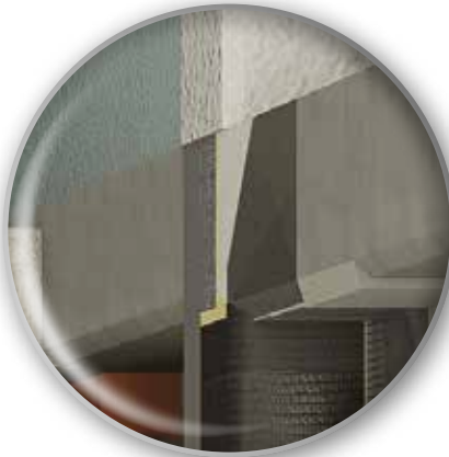
Localised strengthening of beam-pillar joints using carbon fibre fabrics from the FRP System line (ReLuis)
