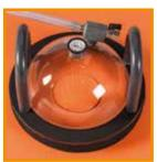
Vacuum Bell Test – joints/patch
