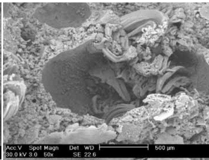
PHOTO 2 - Crystallisation of salts in the macropores of dehumidifying mortar from the MAPE-ANTIQUÉ range
