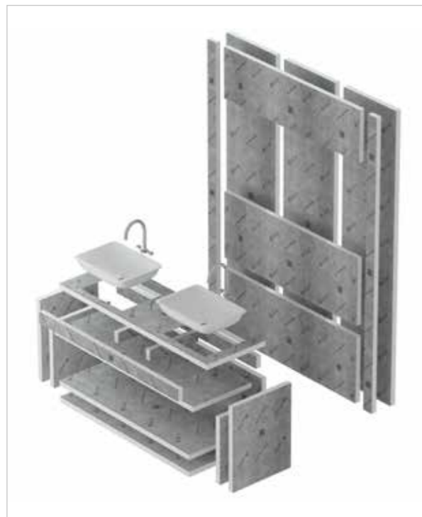
Creating a support surface for washbasins
