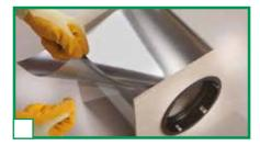
■ MAPESHIELD E, self-adhesive zinc plates applied directly to the external surface of structures to provide galvanic cathodic protection against the corrosion of steel reinforcement.
