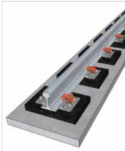
Anchoring and grouting rails for tramlines and/or overhead cranes
