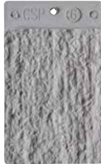
CSP 6: Medium scarification
