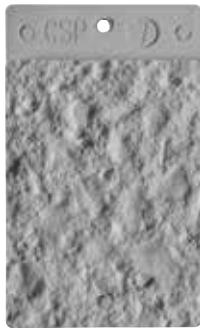
CSP 7: Heavy abrasion blast
