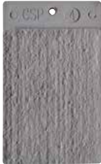
CSP 4: Light scarification
