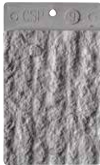
CSP 9: Heavy scarification
