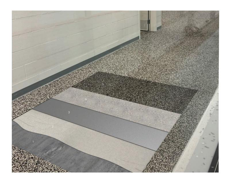
This double-broadcast, decorative epoxy quartz flooring system provides a seamless and non-slip finish using multicolored aggregates. This system provides an impermeable, waterproof, anti-slip finish and does not support growth of bacteria, making it low maintenance. The system is offered with an epoxy cove and a protective polyurethane coating.
