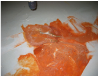
Typical color deviation due to concentrated sulphuric acid attack.
