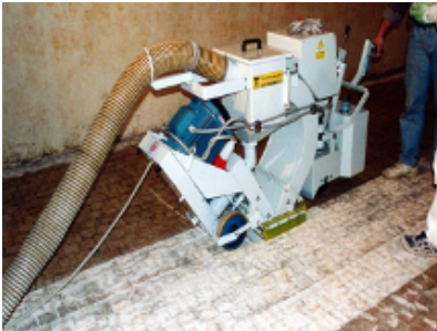
Shotblasting treatment on tiles and old concrete surfaces
