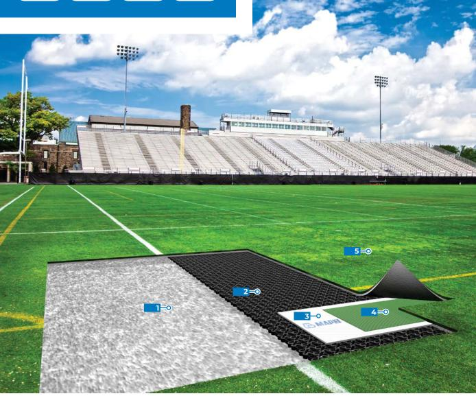
Existing soil treated with Mapesoil 100, or with an aggregate base treated with Mapesoil RD or Mapesoil SR 2 Drainage mat (not required with Mapesoil RD or Mapesoil SR)
