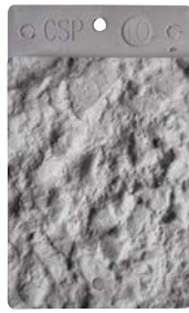
ICRI CSP 10: Concrete breaker and abrasive blasting
