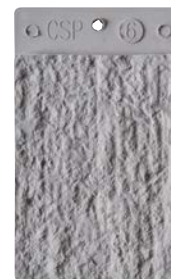
ICRI CSP 6: Medium scarification
