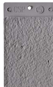
ICRI CSP 5: Medium shotblast
