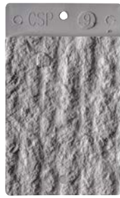
ICRI CSP 9: Heavy scarification
