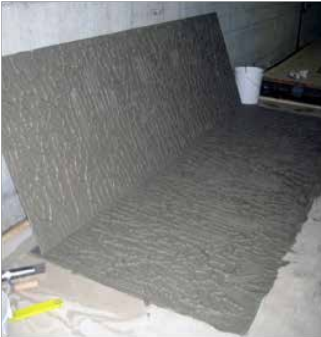
Figure 4: Example of a thin-body porcelain tile with full coverage transfer from tile to substrate
