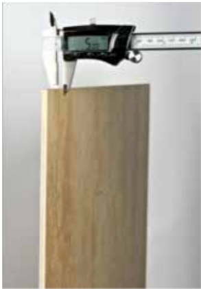
Figure 1: Example of a thin-body, 5 mm porcelain tile
