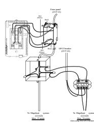
Note: Do not connect neutral wires from different circuits together.
