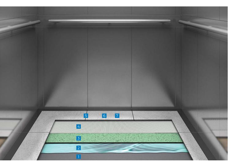
Sheet vinyl is often found in retail settings due to the myriad of design choices and the ease of maintenance. Attention to the installation materials selected will minimize issues such as indents and tears that can be associated with heavy traffic and sheet vinyl flooring.
