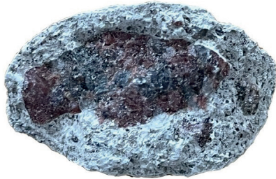
Figure 5_ Extreme closeup of a particle after RE-CON ZERO EVO and RE-CON DRY WASHING process. The cementitious paste has formed a hardened shell around the core stone particle. The grey paste represents on average 30-36% acid soluble content by weight, i.e. material open for potential recarbonation.
