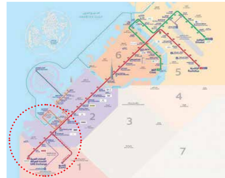
The new Route 2020 is an extension to the Red Line of the Dubai metro system and runs for 15 km from the city to the Expo 2020 Dubai site.
