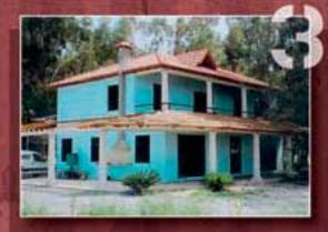
decided to buy a number of used containers and combine them in a two level structure, opening windows and doors at the appropriate places. By the time the containers were put together in the desired order, extruded polystyrene panels were used for external thermo-isolation by fixing them in the outer sides of the containers.
