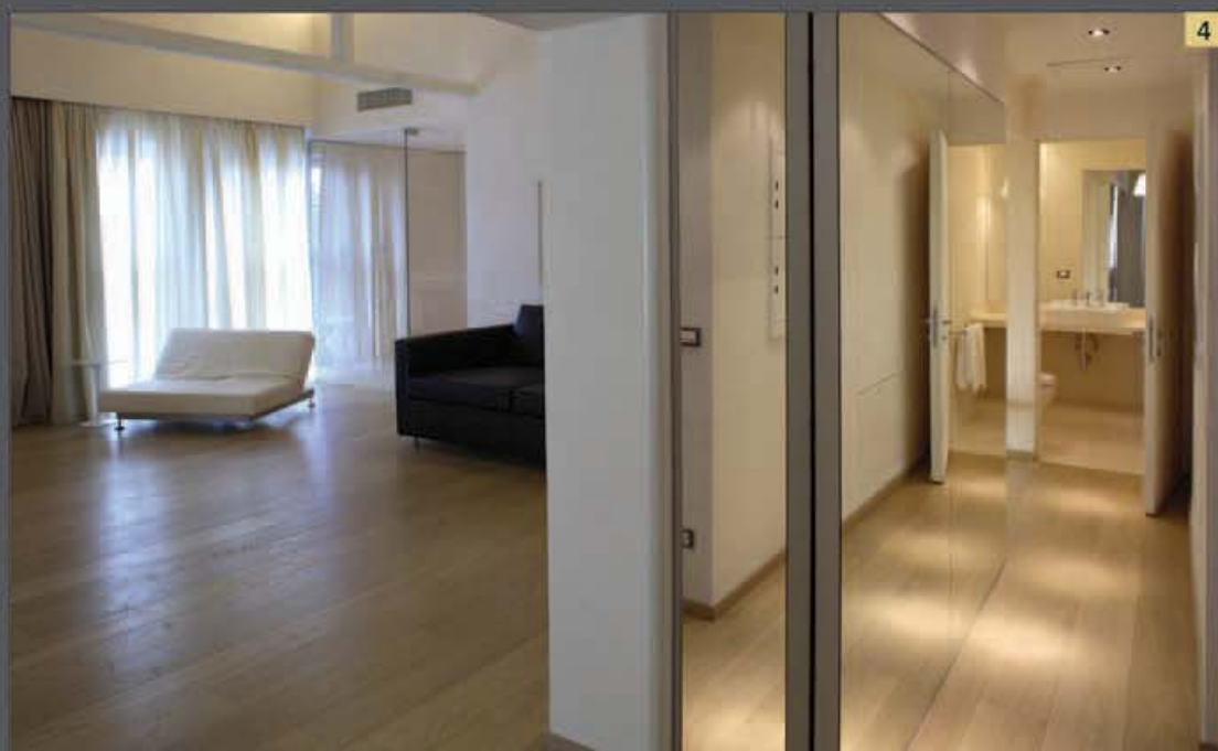
Photos 3 and 4. In the spacious presidential suite about 250 m 2 of clear-coloured oak parquet were laid using Ultrabond P902 2K.
