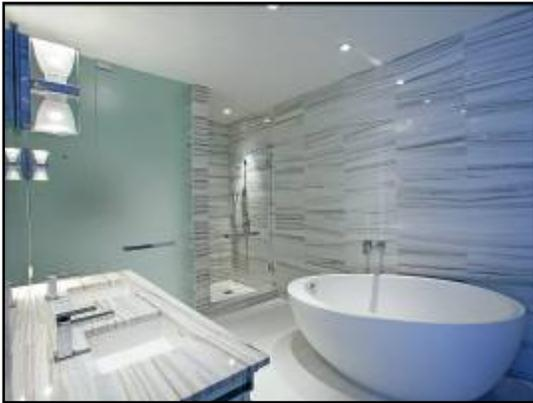
In the bathrooms, the luxury theme continued with the installation of 12" x 24" Cipollino marble tiles on all the walls. Before setting these tiles, the installers applied *Mapelastic HPG*, a ready-to-use liquid waterproofing and crack isolation membrane from MAPEI. Grouting was done with white
