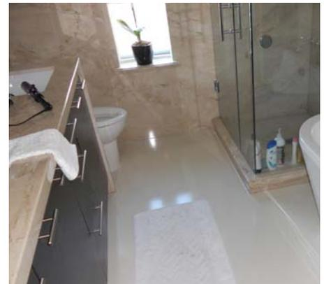
due to the layout of the unit. Once the Ultratop cured for a day, it was buffed and subsequently sealed with an acrylic sealer. Several coats of floor wax were then used to form a protective sacrificial layer. The floor turned out amazingly well and gave the home owner the exact look she was trying to achieve.
