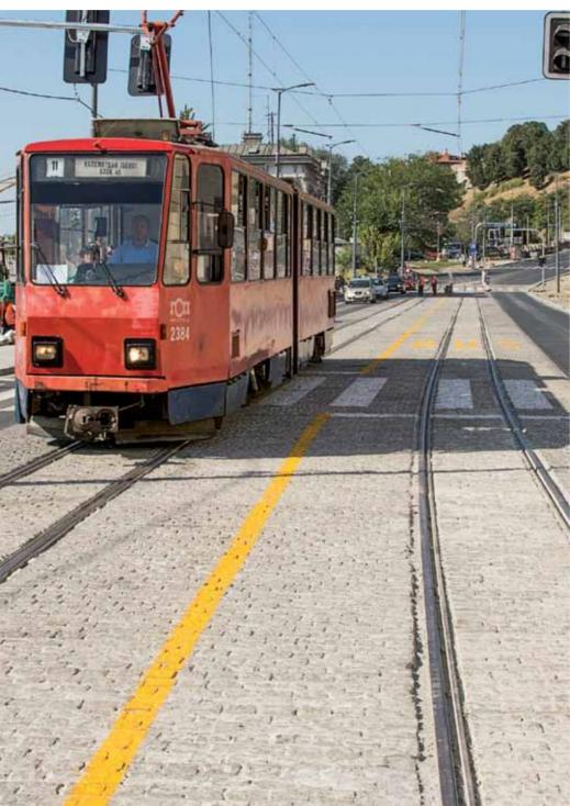
RENOVATION OF THIS ROAD IN THE CENTRE OF OLD BELGRADE INCLUDED THE INSTALLATION OF STONE PAVING IN THE ZONE TO BE USED BY THE CITY TRAM NETWORK
