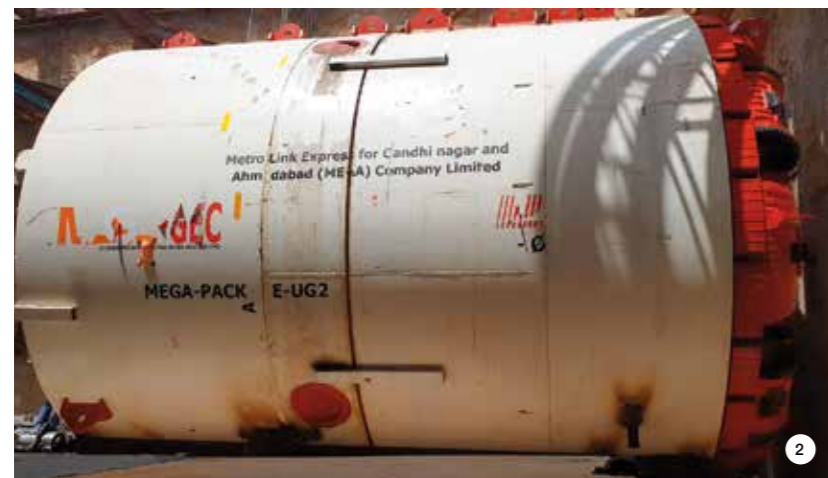
1. Internal view of one of the tunnels excavated using Mapei underground tunnelling solutions, such as POLYFOAMER FP, POLYFOAMER FLS, MAPEDISP FLS, and MAPEBLOX T. 2. An image of the TBM-EPBM tunnelling machine used to excavate the twin-bore tunnels.
