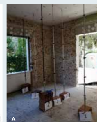
Fig. 2. Area of load test and measuring instruments at ground level in a) pre-strengthening phase b) post-strengthening phase.
