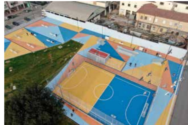
The 5-a-side football pitch was coated with MAPECOAT TNS MULTISPORT PROFESSIONAL, a multi-layered, acrylic resin-based system, which is used for creating polyfunctional sports surfaces with high resistance to wear, UV rays and atmospheric agents.
