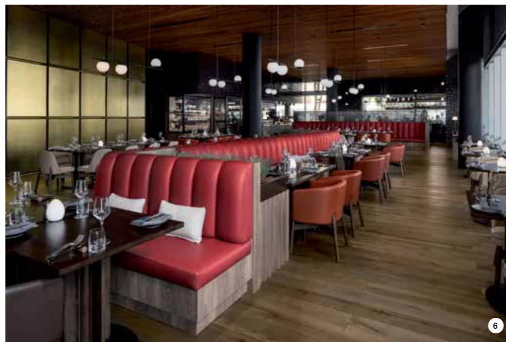
5. In the bathrooms the screeds were made of TOPCEM, before waterproofing the substrates with MAPEGUM WPS. 6. Wooden floors were installed in the restaurant and foyer areas using ULTRABOND ECO S955 1K, one-component, solvent-free, sililated polymer adhesive.
