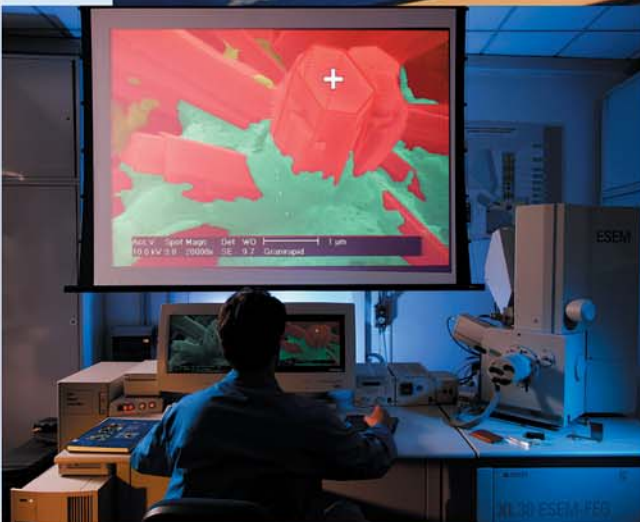
Images portraying the Philips XL 30 ESEM-FEG "environmental" scanning electron microscope.
