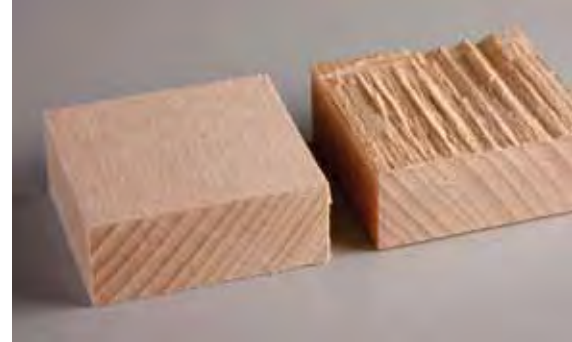
FIG. 2. A new test sample and a broken test sample after applying a compressive shear load with a dynamometer.
