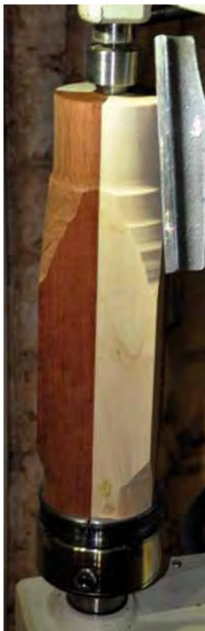
FIG. 1. Using a lathe to turn a pepper mill formed by bonding two types of wood.
