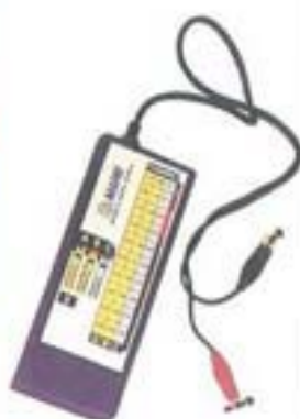
PHOTO 2 Carbide hygrometer for an absolute measurement of humidity, and below the MAPEI electronic hygrometer
