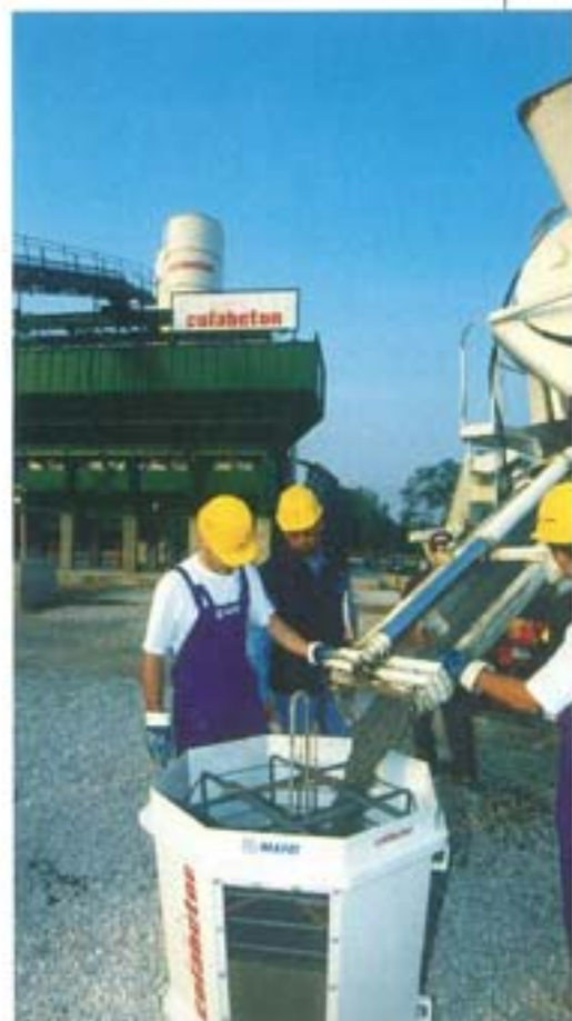
Fig. 2. On-site evaluation of self-compactability.
