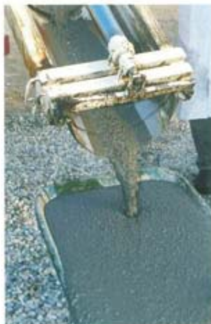
Fig. 1. Self-compacting concrete before quality control.
