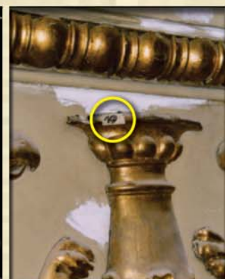
Sample 19 was taken in a point where the decorations were probably the original ones from the start of the 19 th century.
