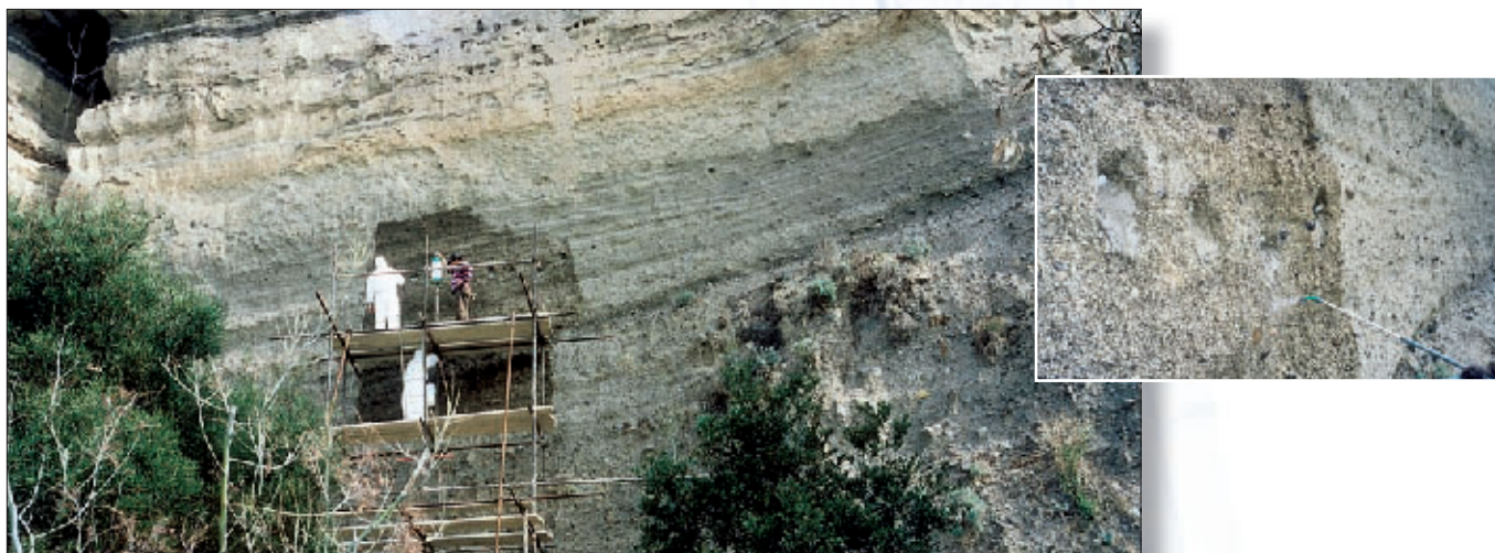
Photo 1. The application of Primer 3296 was tested at Monte di Procida (Province of Naples, Italy).
