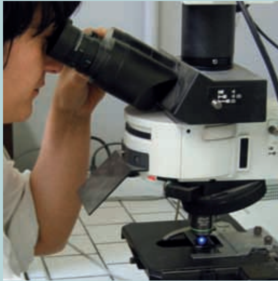
Left: a stage in controlling the bituminous layers and studying their properties under a microscope.
