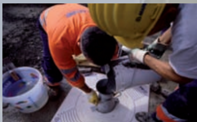
Sequence of the various phases of the slump-flow test, which indicates the consistency of the concrete.
